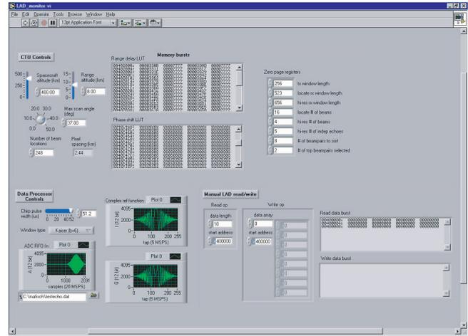
Figure 7: Graphical user interface (GUI) for the PR-2 test fixture. Features include a programmable lookup table interface for radar range delays, a chirp waveform generator, and a module for programming the matched filter coefficients for pulse compression.
